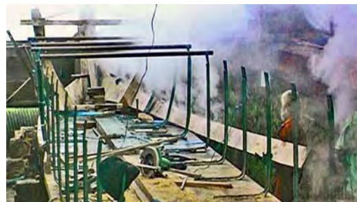
Richard (lost in the steam) and Phil position the second plank.
