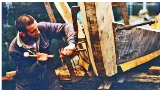
Richard secures the plank to the stem post.
