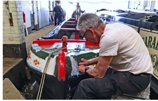
Norman Townsend repairing rot behind Raymond's stern post
