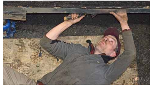
Scott from Bates Boatyard fits the chine shoe plating 7 April 2017. Picture: Diana Golder
