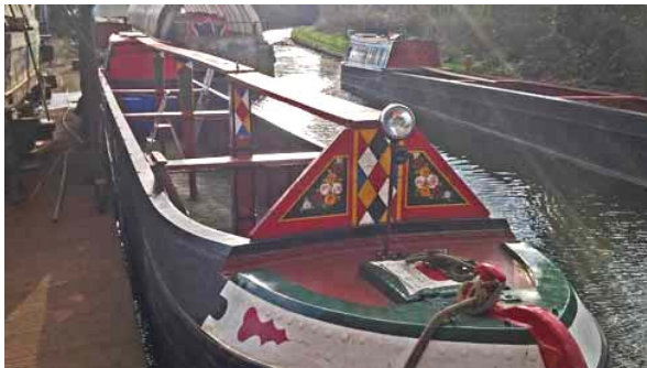
Top: Detail of new gunwales and deck beam, 27 Sep 2017 Bottom: Ready for side cloths, 23 Nov 2017
