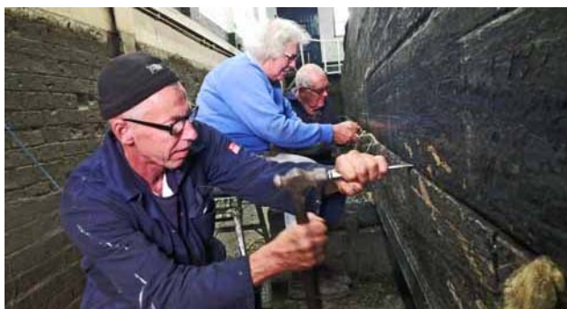
Norman Townsend, Diana Golder and Mike l'Anson caulk the seam between the first and second planks, 3 October 2018
