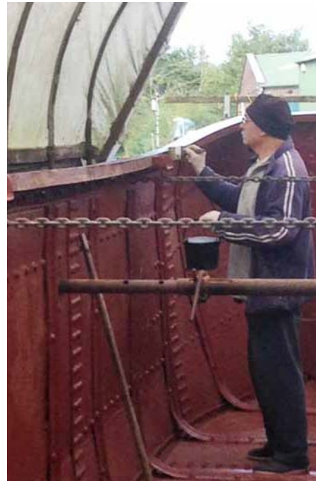
Chris M Jones treats the gunwales with wood preservative, 7 Oct 2017. Picture: Chris R Jones
