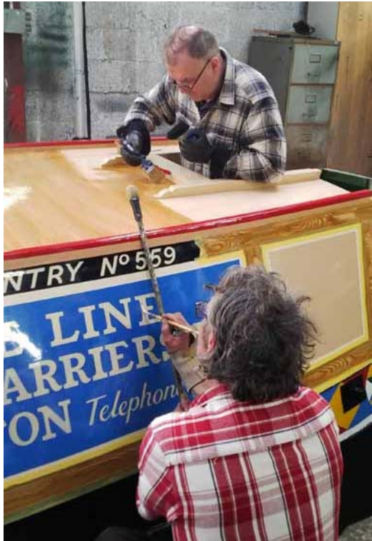
Top left: FoR's Caroline Brudenell undercoats the roof, 23 March 2017 Right: FoR's Peter Copeland scumbles the roof while Alan Baillie completes the lettering, 1 April 2017 Bottom left: the finished cabin, 1 April 2017
