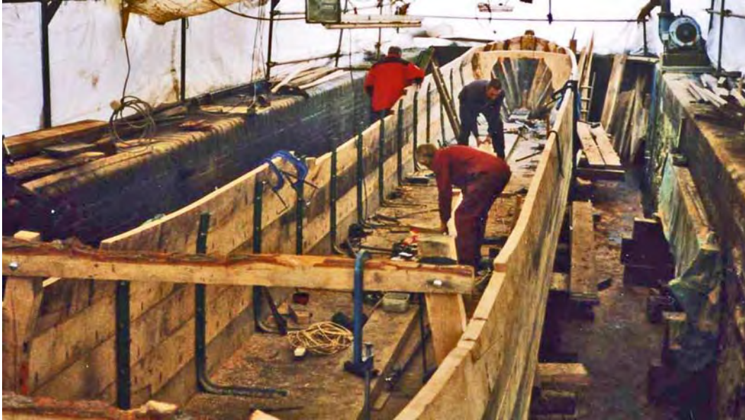
Raymond being rebuilt in the dry dock at Tardebigge by Phil Babb and Richard Clapham, February 2000. The full story will be told in the next issue of FoR News . Picture FoR collection
