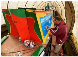
Other jobs completed by Saturday 1st April include repairing and priming the cabin gunwales, painting the engine room bulkhead, undercoating the cabin doors and bulkhead, painting the stern cants, and touching up the tunnel bands.
